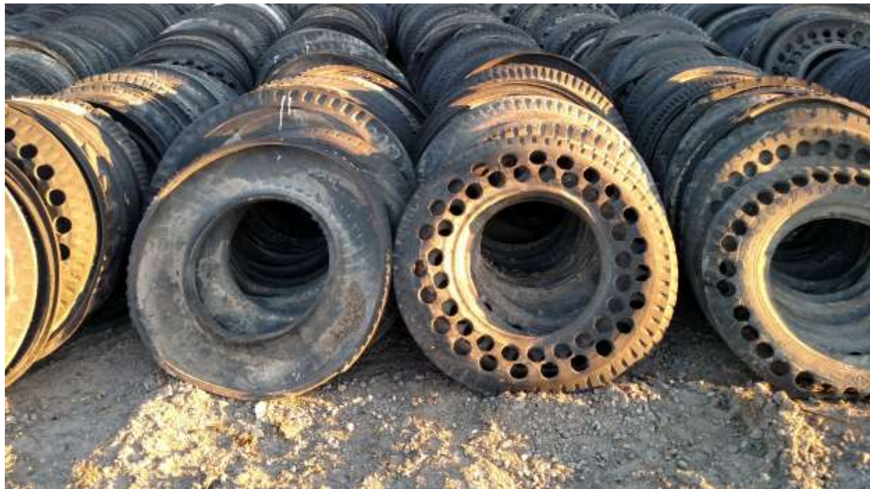
Image 2: Side walls that have been halved and holes drilled in them. The farmer paid approximately $2.00 per side wall.
